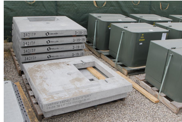
SINGLE PHASE UG TRANSFORMERS
